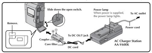
**TONNECT DC CORD TO CAMCORDER**Insert the coupler of the provided DC cord into
